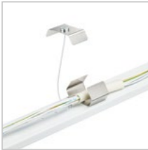
The safety clips with safety cable allow easy installation. First hook in, connect electrically, then place the light panel in the bar
