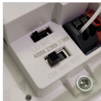
The light colour and luminaire luminous flux can be easily adjusted on site using two mini switches.
